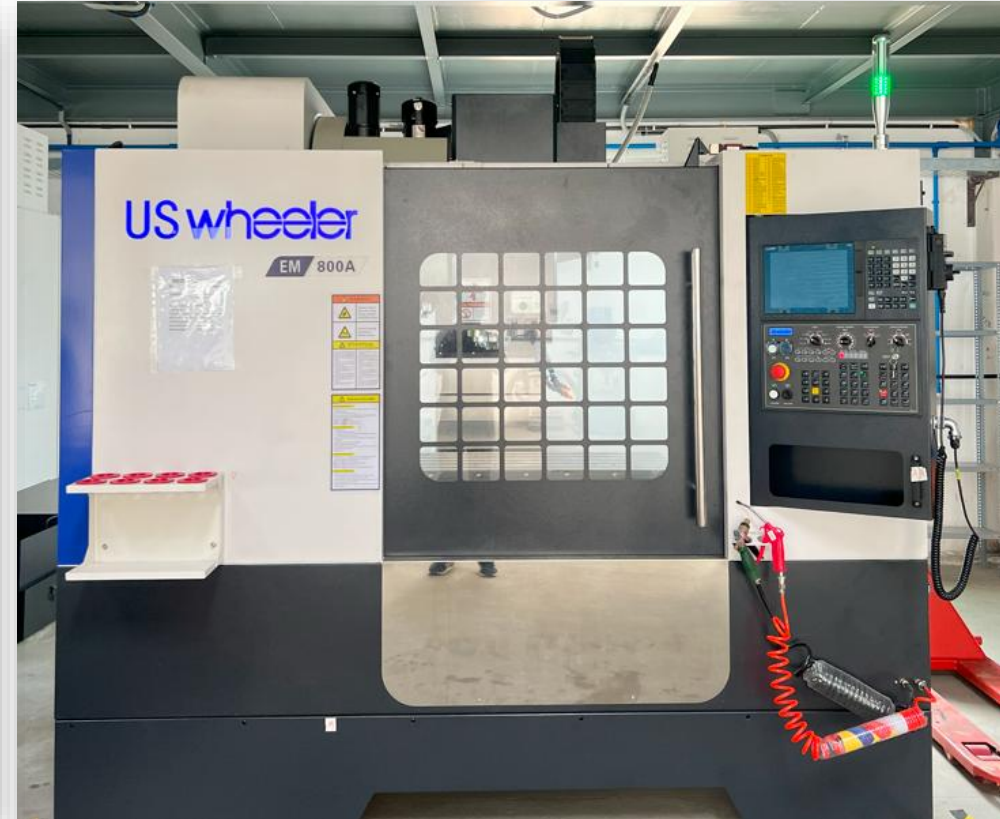
Equipment: Vertical Milling Centre Model: EM800A Bed Size: X-800, Y-500, Z-500 mm Tool Changer Type: ATC with 24 Tools Quantity: 02
