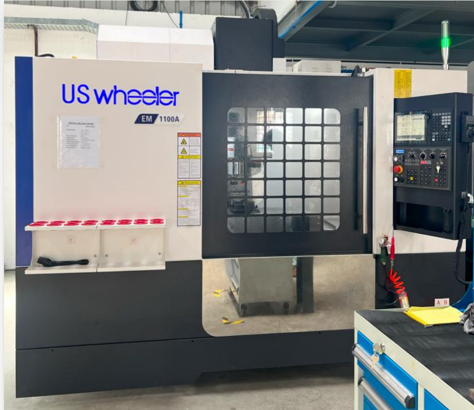
Equipment: Vertical Milling Centre Model: EM1100A Bed Size: X-1100, Y-600, Z-600 mm Tool Changer Type: ATC with 24 Tools Quantity: 01
