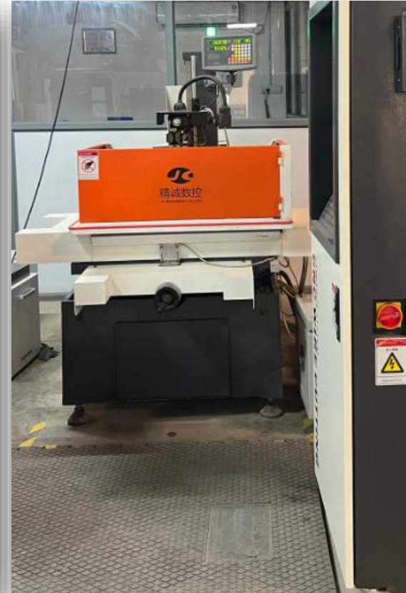
Equipment: Fast Wire Cut Model: JC-4555B Max. Thickness of Job: 400mm Accuracy: 0.012mm
