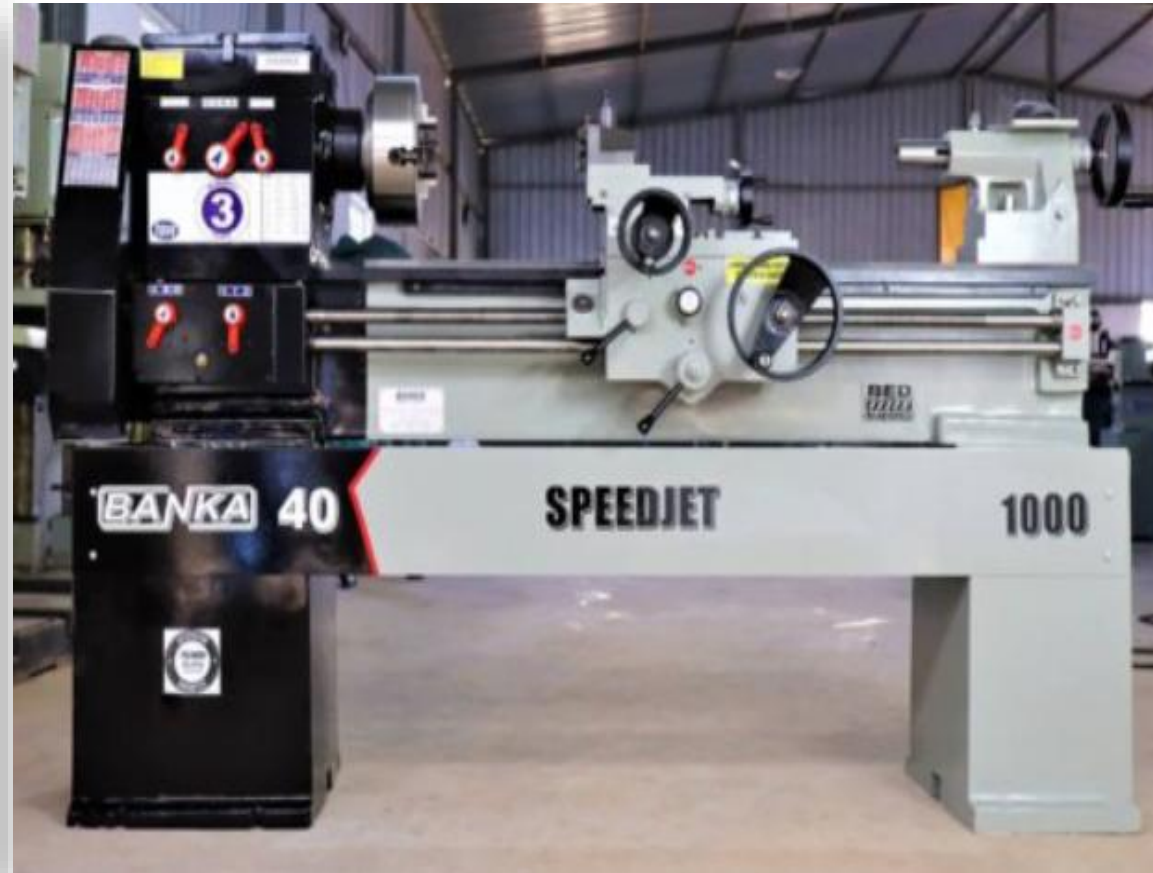
Lathe Machine Model: 40-1000 Max Length: 1000 mm Max Dia: 250 mm Quantity: 01
