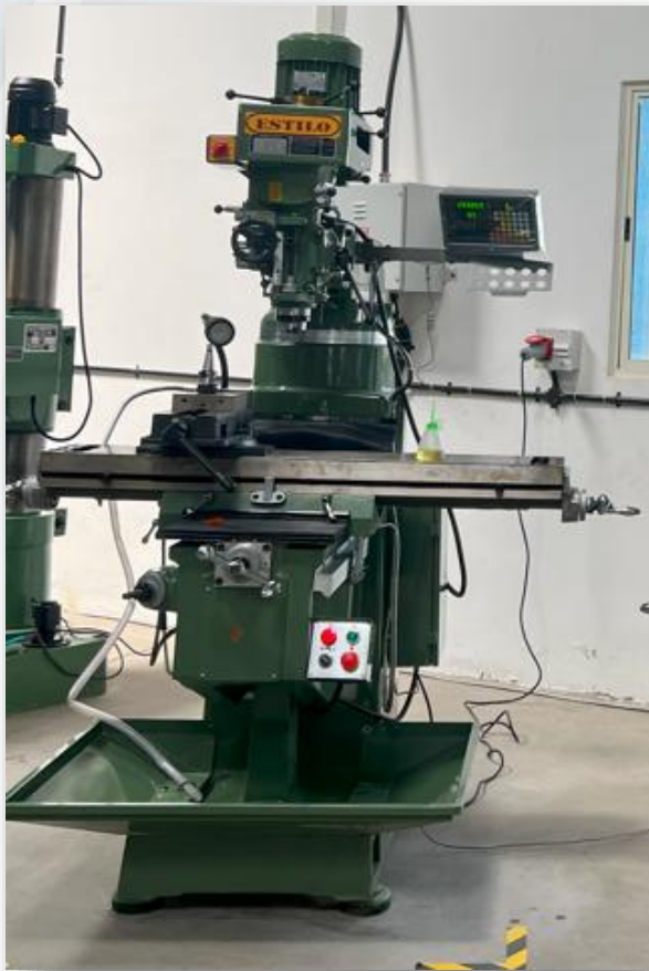
Vertical Milling Machine Model: M4A Table Size: 1370 x 254 mm Ram Travel: 510 mm Quantity: 02
