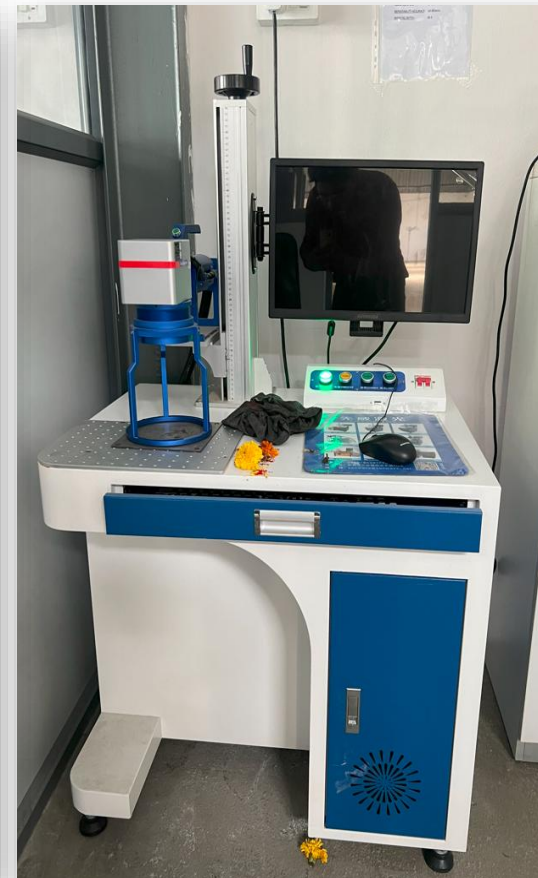
Fiber Laser Engraving M/C Model: SW-QXGQ30A Marking Range: 300 X 300 Quantity: 01
