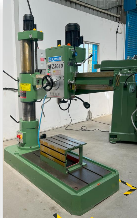
Radial Drilling Machine Model: Z3040 Arm Length: 1300 mm Spindle Travel: 200 mm Quantity: 01
