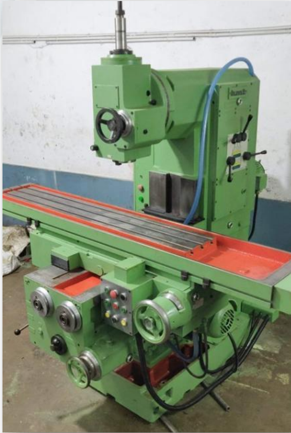
Vertical Milling Machine Model: F1 Table Size: 1370 x 254 mm Ram Travel: 600 mm Quantity: 01
