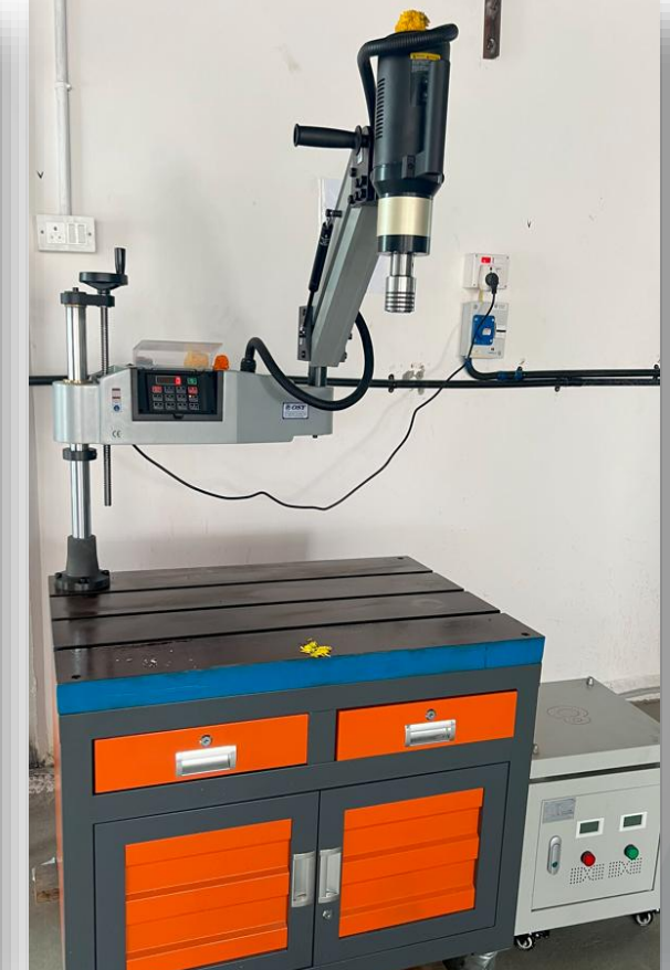
Auto Tapping M/C Model: M36 Tapping Range: M6-M36 Quantity: 01
