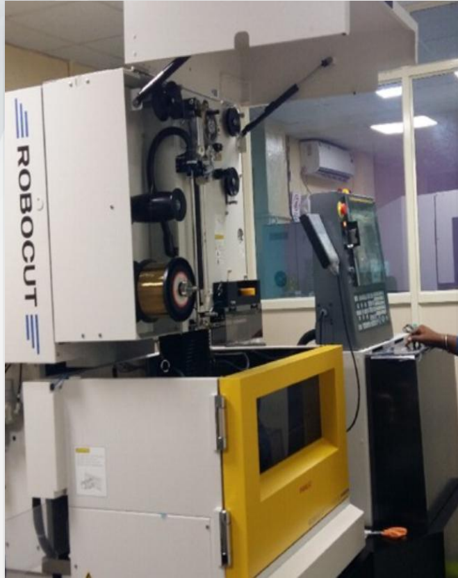
Equipment: Fanuc Robo cut Model: α-C400iC Max. Thickness of Job: 255mm Positioning Accuracy: 0.0001mm
