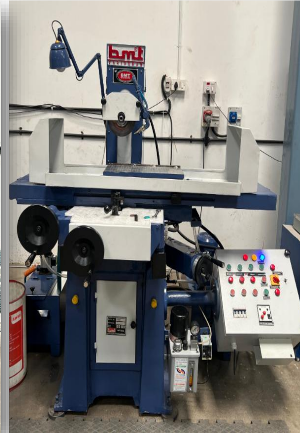
Equipment: BMT Hydraulic SG Model: AH-500 Job Size: 250 x 500 Accuracy: 0.002mm Quantity: 01
