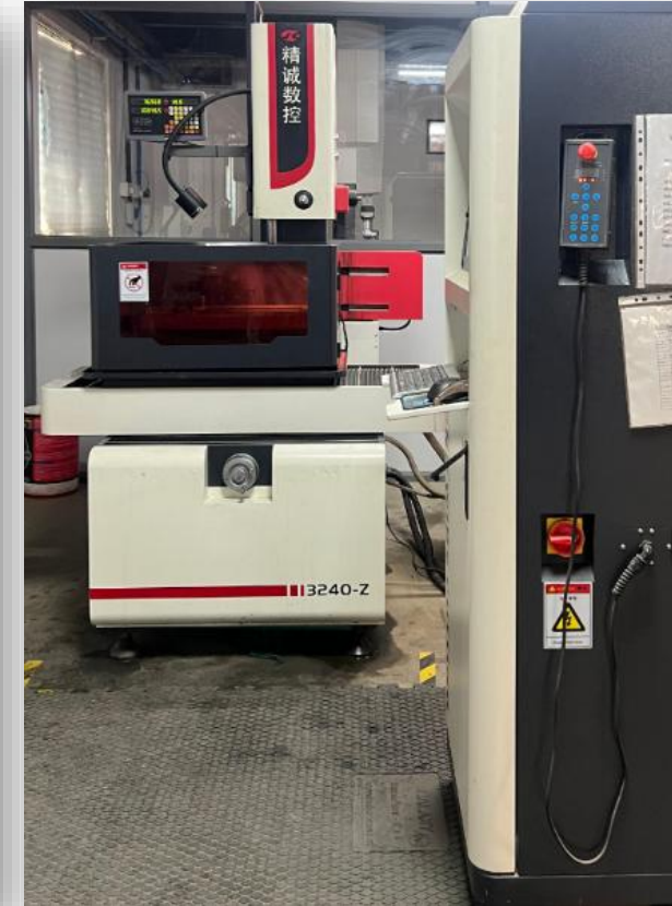
Equipment: Medium Wire Cut Model: JC-3240Z Max. Thickness of Job: 300mm Accuracy: 0.01mm
