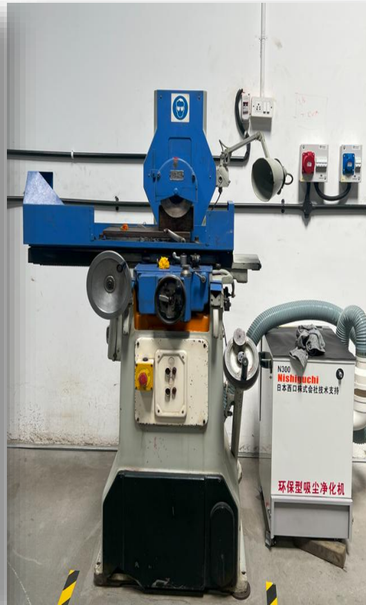
Equipment: Hydraulic SG Model: JONES- SHIPMAN (UK) Job Size: 400 x 300 Accuracy: 0.002mm Quantity: 01
