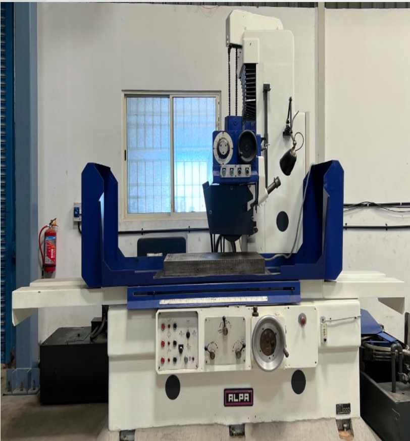
Equipment: Wet Surface Grinding Machine Model: ALPA RT1000 (ITALIAN) Job Size: 1000 x 500 Accuracy: 0.005mm Quantity: 01
