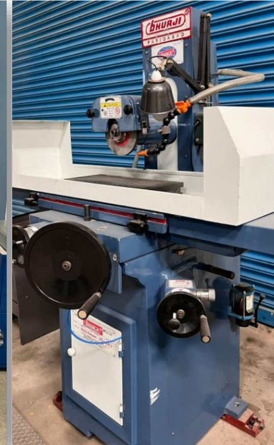
Equipment: BMT Manual SG Model: AH-500 Job Size: 250 x 500 Accuracy: 0.002mm Quantity: 01
